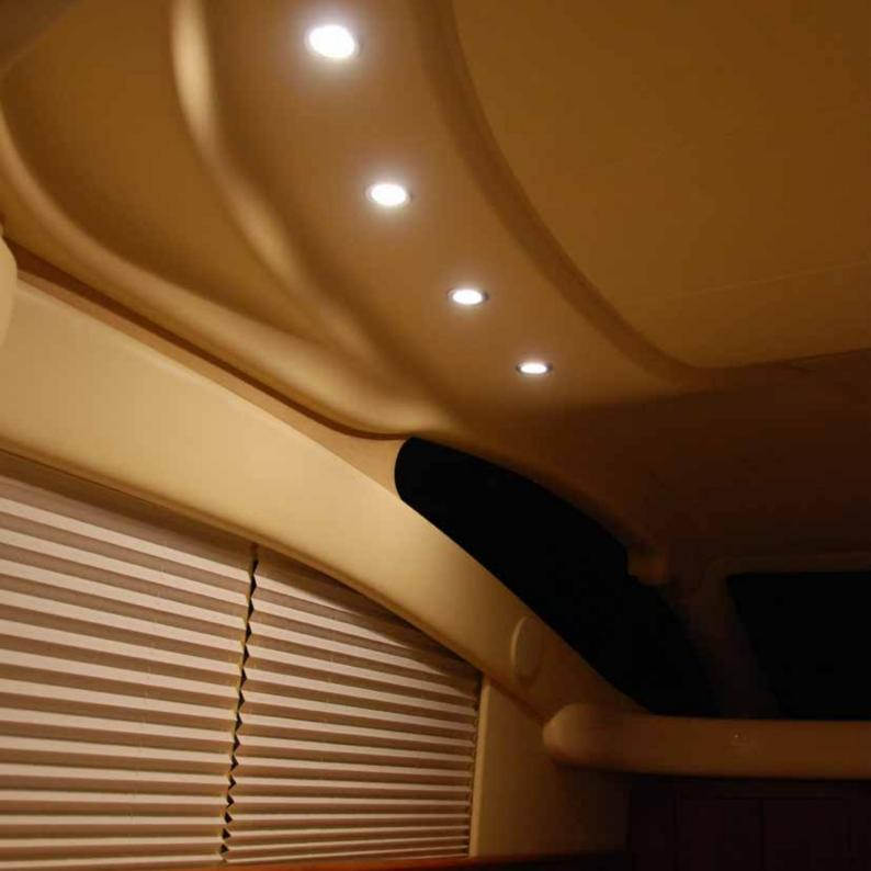
Compact LED light with electronic driver built-in waterproof anodized aluminium casing designed by using 2, 3 or 6 high-power LEDs with built-in microprocessor which enables network connections and remote control with digital dimming.
